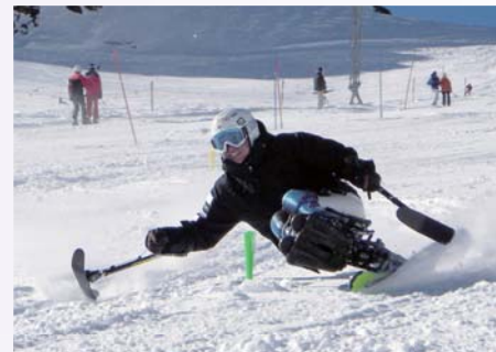
Chair Ski Shock Absorbers for Disabled Skiing “滑雪椅用减震器”
