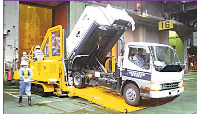
Self-propelled waste checker conveyor 自带动力传送带式垃圾投入检查机
